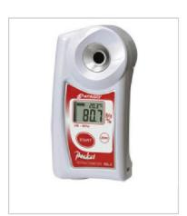
Since the measurement range of PAL-2 is Brix 45.0 - 93.0%, it can measure various high concentration samples such as jam, marmalade, jelly, honey and concentrated juice. The International Protection class of PAL-2 is IP65, so it can clean thick samples under running water. If you measure boiling jam or marmalade, we recommend PAL-H
