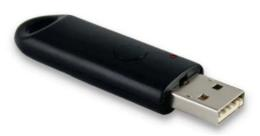
This low cost data logger measures and stores up to 4,080 temperature readings over a -10 to +50 °C (+14 to +122 °F) measurement range with a fixed 30 minute sample rate and a battery life of 1 month continuous use.
