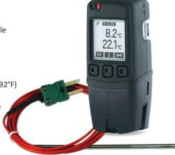
This standalone data logger measures and stores more than 250,000 temperature readings from two K, J or T-type thermocouple probes at a resolution of 0.1°C (0.2°F). It comes supplied with two K-type thermocouples capable of measuring from 0 to 200°C (32 to 392°F).
