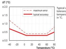
Typical and maximal tolerance for temperature sensor
