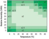
Typical accuracy of relative humidity measurements given in %RH for temperatures 0 to 80°C.
