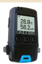
The EL-GFX-2 standalone USB data logger measures and stores up to 252,928 temperature and humidity readings over a -30 to +80°C (-22 to 176°F) and 0 to 100%RH range at a resolution of 0.1°C and 0.1%RH.
